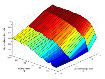
Fig. 6. Simulation results of maximum SNR of LC  $\Sigma\Delta$  modulators having different undersampling factors and finite Q factors.
