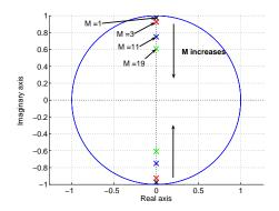
Fig. 5. Pole location of the LC  $\Sigma\Delta$  loop gain,  $G_c(z)$ , for different undersampling factors, M, and a Q factor of 30.
