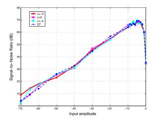
Fig. 7. Simulation results of  $4^{th}$  order DT and undersampled LC  $\Sigma\Delta$  modulators using different values for  $\lambda$  (table I).
