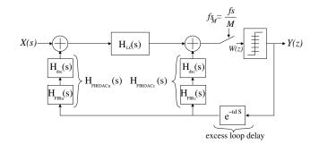
Fig. 1. LC bandpass  $\Sigma\Delta$  modulator with an undersampling factor M.
