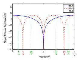
Fig. 2. NTF of LC  $\Sigma\Delta$  modulators having odd undersampling factors. NTF notch is located at multiples of  $\frac{f_0}{M}$ .
